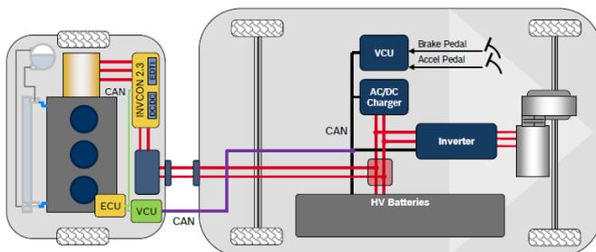
Vehicle diversity is managed by adding a "CAN Merger Box" along with the high voltage junction box in order to select and reformat the vehicle's CAN messages into a vehicle independent format. When the energy module carries a battery, or a fuel cell, a DCDC power electronics module will provide the necessary voltage adjustments. When the energy module carries an ICE generator, the generator's output is equipotential with the vehicle's battery.
